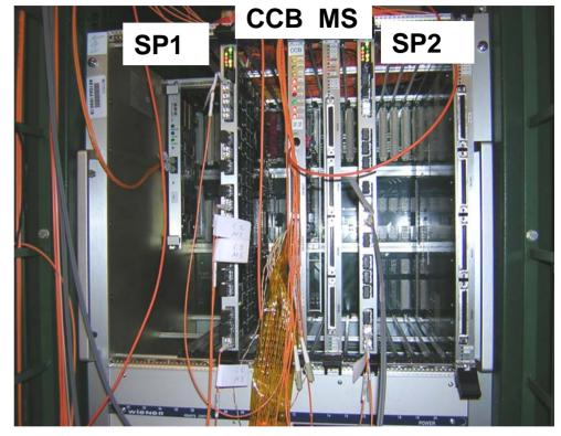
Have tested up to 3 peripheral crates (~3 EMU disks  $\times$  60°) with up to 2 SP's (2×60° sectors)
