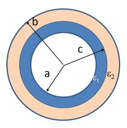
The space in between the spheres is filled with two spherical shells made of *different* insulators, so that
