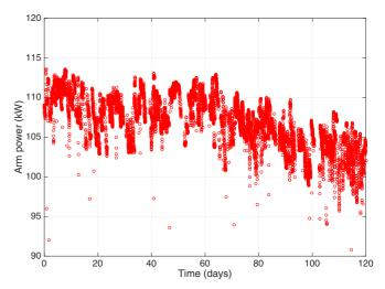
FIG. 2. Optical power resonating in the LIGO Livingston interferometer (L1) during the first science run. The power was fluctuating by a few percents, and slightly decreased by the end of the run due to the drift of the input power.
