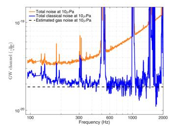
FIG. 4. Measurement of the gas phase noise in the Livingston detector when the nitrogen pressure was increased up to 10  $\mu$ Pa.
