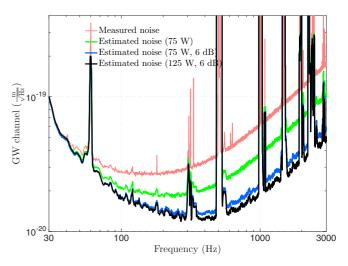
FIG. 5. Estimated noise spectra of LIGO interferometers for future science runs when the input power is increased and squeezed states of light are introduced.
