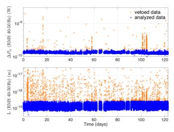
FIG. 8. Data quality cut. The quality of the data is estimated based on the rms of the signal computed between 40 and 50 Hz. Red points are subtracted from the analysis.
