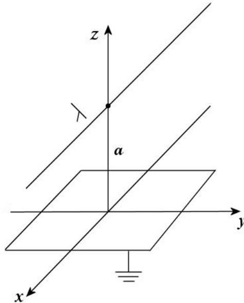
Let's orient the axes so that the conducting plane is in the  $xy$  plane, and the wire runs parallel to the  $x$  axis and directly above it, intersecting the  $z$  axis at the point  $z = a$  as shown in the figure.
