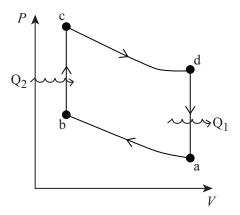
Consider an ideal gas as the working substance for the "Otto" cycle that is sketched on the P vs. V plot. As you may recall, a-b and c-d are adiabatic processes, while b-c and d-a are isochoric processes.
