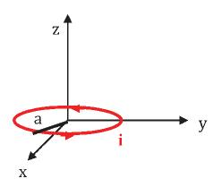
A circular current loop of radius a lies in the x-y plane (z = 0) with its center pierced by the z-axis as shown in the figure. The current i moves in the counter-clockwise direction in the x-y plane.
