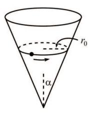
A particle slides on the inside surface of a frictionless cone. The cone is fixed with its tip on the ground and its axis vertical. The half-angle at the tip is  $\alpha$  (see the figure). Let r(t) be the distance from the particle to the vertical axis, and let  $\theta(t)$  be the angle around the cone.
