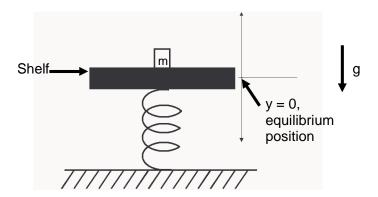
(negligible mass compared to the shelf) is laid on the shelf at time t=0 when the shelf is at its lowest position i.e. y=-30 cm (the particle is light enough such that it does not affect the simple harmonic motion of the shelf).
