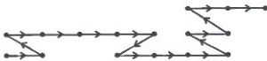
Figure 1. A collection of links representing a simplified model of a rubber band. The links lie in the +z and -z directions. Some of the links are drawn at an angle so the arrangement may be seen more clearly. Figure from R. Bowley and M. Sánchez, Introductory Statistical Mechanics , Oxford Science Publications.
