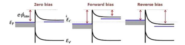
Schematic energy level diagram showing a metal/semiconductor interface at zero bias, forward bias (V > 0) and reverse bias (V < 0).  $E_F$  is the Fermi energy of the metal,  $\Phi_{SBH}$  is the Schottky barrier height, and  $E_C$  and  $E_V$  are respectively the conduction and valence bands of the semiconductor.
