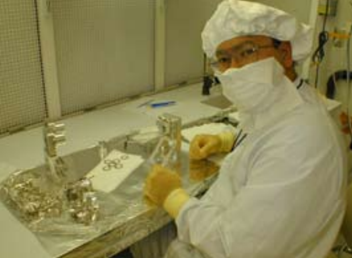
UF research scientist Malik Rakhmanov assembles a Brewster polarizer on a laminar flow bench for installation into the LIGO Hanford 2 km long interferometer. Many of the optical components of the interferometer are located in a high vacuum system placing stringent requirements on cleanliness.
