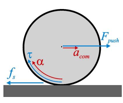
•If the c.o.m. moves with constant velocity, and the wheel rotates with constant angular speed  $\omega = v_{com}/R$ , then there are no net forces on the wheel.
