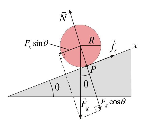
Use: torque =  $I \alpha$  $R \times F_{g} \sin \theta = I_{P} \alpha$  $a_{com} = -\alpha R$ Thus:  $MR^2g\sin\theta = -I_Pa_{com}$  $I_P = I_{com} + MR^2$  $g\sin\theta$ a<sub>com</sub>  $1 + I_{m} / MR^{2}$
