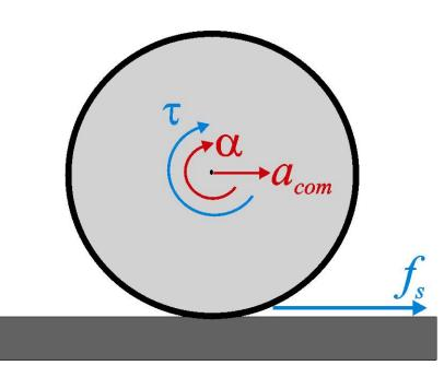
•If the c.o.m. moves with constant velocity, and the wheel rotates with constant angular speed  $\omega = v_{com}/R$ , then there are no net forces on the wheel.
