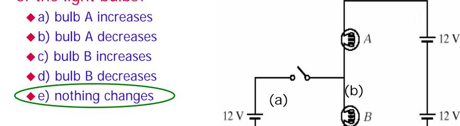
Before: Potential at (a) is 12V, but so is potential at (b) because equal resistance divides 24V in half. When the switch is closed, nothing will change since (a) and (b) are still at same potential.
