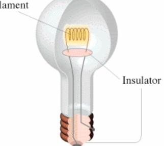
$P = I^2 R = V^2/R$ , so 100W bulb has <sup>1</sup>/<sub>4</sub> the resistance of the 25W bulb and carries 4x the current.
