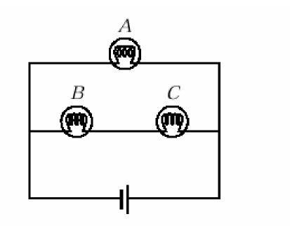
→The three light bulbs in the circuit are identical. What is the brightness of bulb B compared to bulb A?
