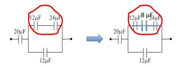
Next step: 8 and 12  $\mu F$  capacitors are connected in parallel  $C=8+12=20~\mu F$
