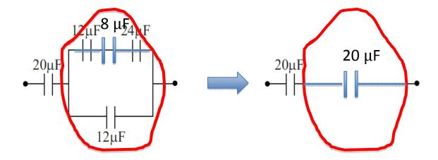
The last step: the two 20  $\mu F$  capacitors are connected in series. The equivalent capacitance is 10  $\mu F$ .
