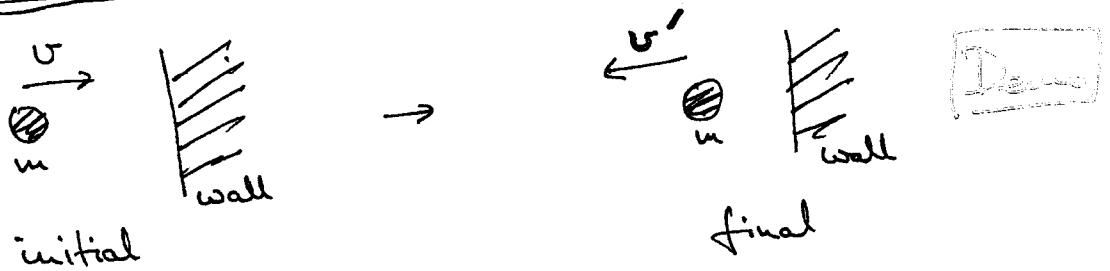
equation ④  $\Rightarrow m v + M \cdot 0 = -m v' + M V$
