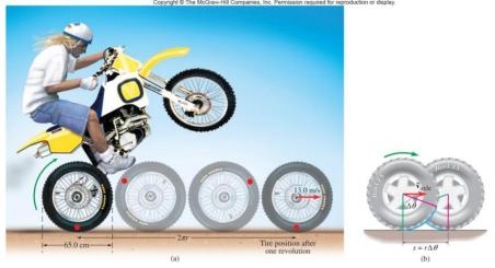
If the wheel rolls without slipping, the axle of the wheel moves with a speed of v given by
