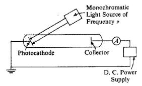
In this apparatus, the photocathode and the collector are made from the same material. The potential V of the collector, measured relative to ground, is initially zero and is then increased or decreased monotonically. The effect is described by Einstein's photoelectric equation
