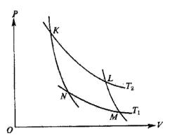
95. In the cycle shown above, KL and NM represent isotherms, while KN and LM represent reversible adiabats. A system is carried through the Carnot cycle KLMN, taking in heat Q2 from the hot reservoir  $T_2$  and releasing heat  $Q_1$  to the cold reservoir  $T_1$ . All of the following statements are true EXCEPT:
