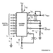
$V_I$  and  $I_1$  apply to inputs A1-A8.
