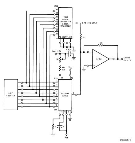
FIGURE 4. Relative Accuracy Test Circuit (Note 8)
