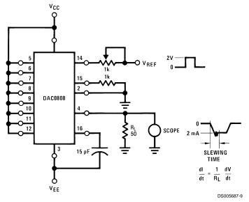
FIGURE 6. Reference Current Slew Rate Measurement (Note 8)
