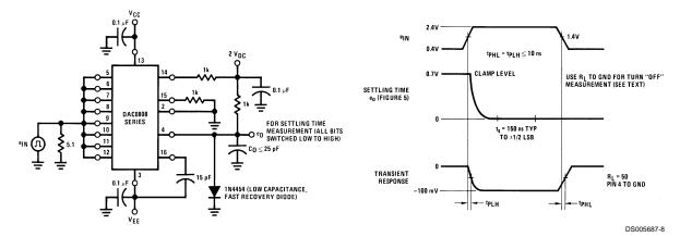
FIGURE 5. Transient Response and Settling Time (Note 8)
