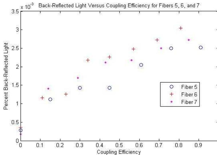
Figure 10: Plot of percent back-reflection versus coupling efficiency.
