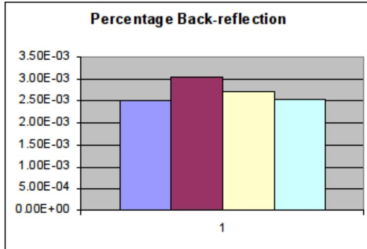
Figure 7: Bar graph of the percent back-reflection. Fiber 5 is in blue, fiber 6 maroon, fiber 7 peach, and fiber 8 teal.
