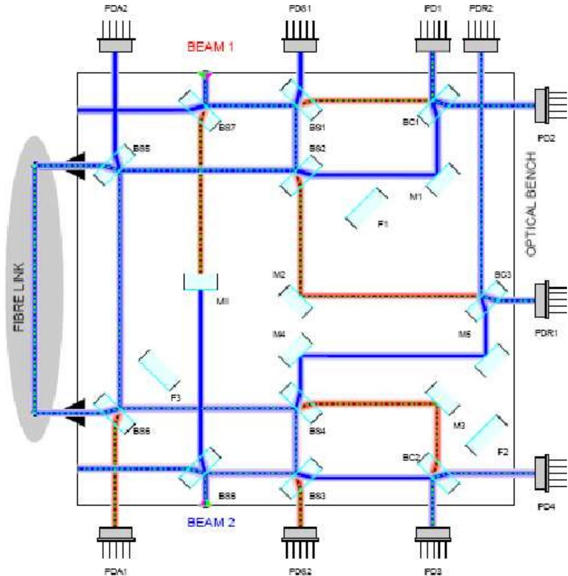
Figure 1: The nonreciprocal phase noise setup.
