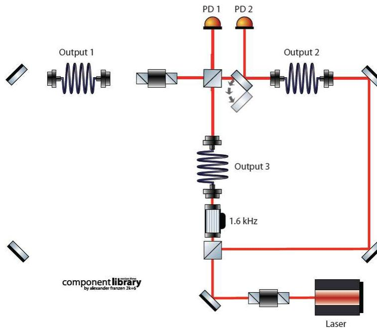
Figure 12: Set-up for measuring attenuated back-reflected light.
