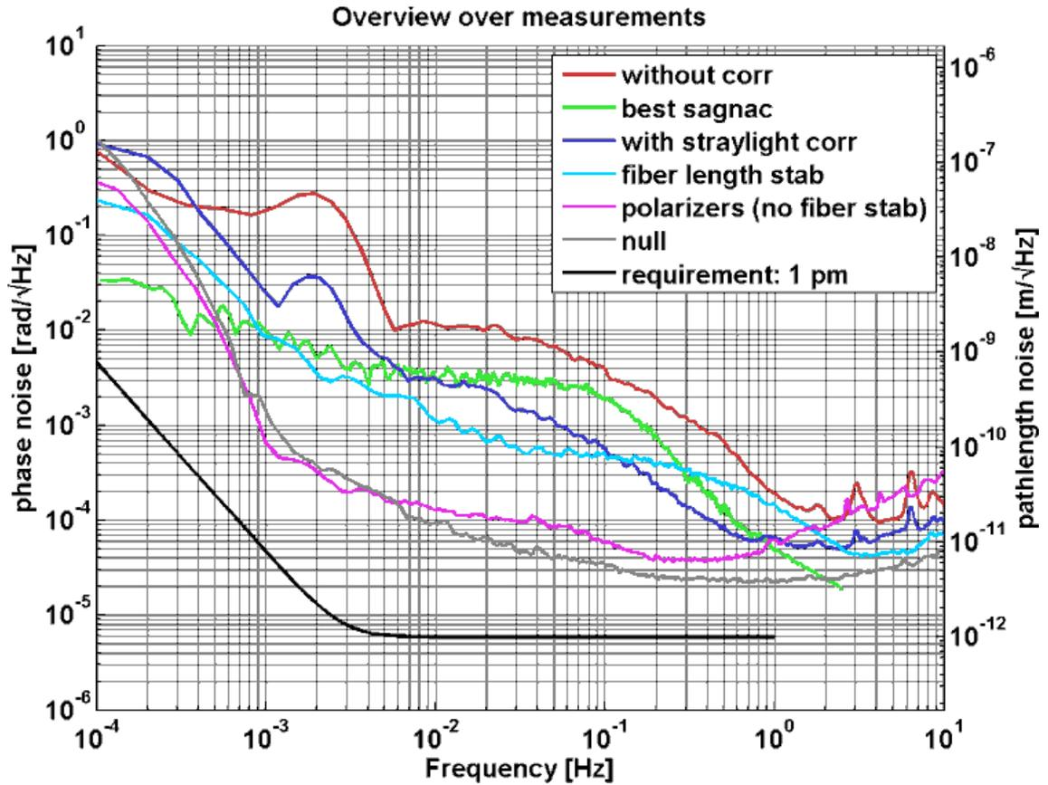
Figure 2: Noise levels for various nonreciprocal phase noise measurements.
