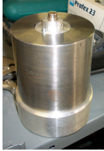
Figure 2.4: The 5 kg mass with the magnet attached
