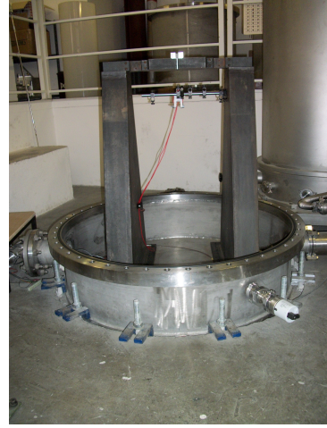
Figure 2.1: Steel structure used to suspend the fiber
