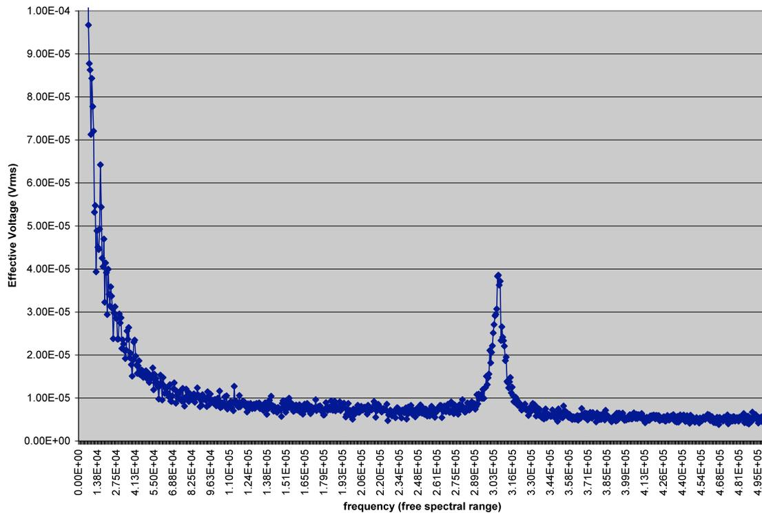
When we calculate the laser frequency change in comparison to the amount of error signal being read, the results show that there is 1 Volt of error signal read for every 425.2 kHz of residual laser frequency noise that shift out of resonance.
