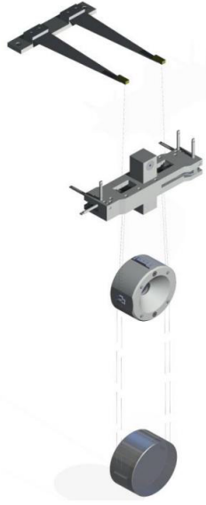
Figure 5: The triple suspension system used for the reference cavity mirrors of the 10m prototype. This is very similar to the suspension system for the main interferometer mirrors. The top, middle, and bottom masses are the initial mass, the intermediate mass, and the mirror, respectively. The upper stage consists of two cantilever springs to suppress vertical motion.
