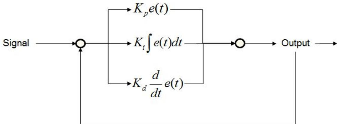
**Figure 8.** Visual representation of the workings of a PID.  $e(t)$  represents the error signal calculated by the PID (as the difference of the desired point to the actual point.) Each  $K$  is the gain of each PID term. Our PID does not explicitly use functions of time, but still is very effective as we shall see.
