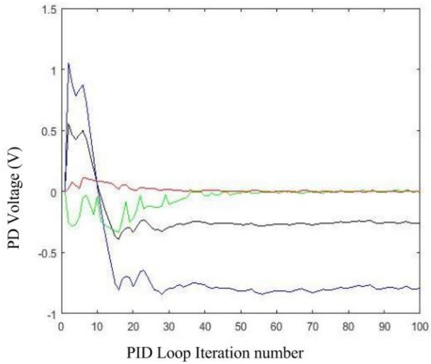
**Figure 9.** PID tuning using only the integral term.
