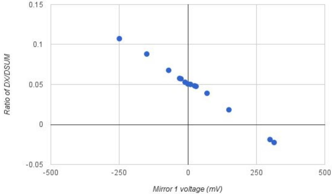
**Figure 7.** Calibration data. Ratio of registered X to SUM voltages across PD2 versus voltage applied on M1. (Note: The D’s in “DX/DSUM”, was for our personal labeling purposes.)
