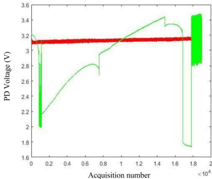
**Figure 12.** Laser stability comparison, green versus red laser. Green laser parameters (LED power, and temperature control were not optimal.) Not shown, but even with optimal parameters, the power fluctuations of the green laser were 2-3 times that of the red laser; leading us to choose the red laser for the duration of the research.
