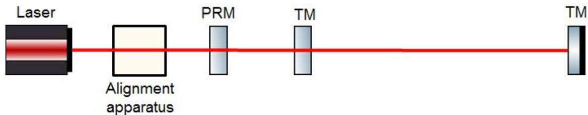
**Figure 2.** Model of CALVA's optical cavity; (essentially one interferometer arm, with a power-recycling mirror.) The alignment apparatus will be placed before the optical cavity, after input laser signal.
