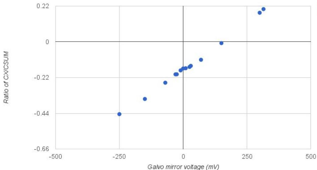
**Figure 6.** Calibration data. Ratio of registered X to SUM voltages across PD1 versus voltage applied on M1. (Note: The C's in "CX/CSUM", was for our personal labeling purposes.)
