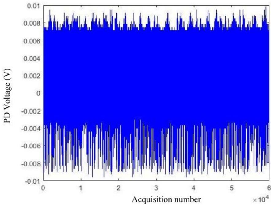
**Figure 5.** PD2 electronic dark noise with calculated center at about 0.7 mV
