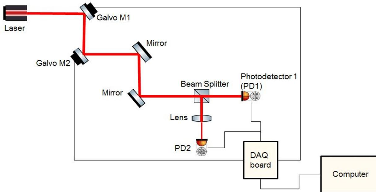
**Figure 3.** Optical alignment system for CALVA. PD1 is sensitive to beam translation and rotation, and PD2 is sensitive to solely beam rotation. A (PID) feedback loop will acquire beam position data from the PDs, and send correction signals to the galvo mirrors to center the beam.
