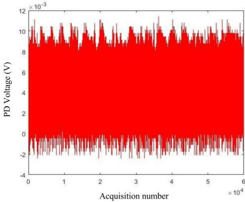
**Figure 4.** PD1 electronic dark noise, with calculated center at about 3 mV.
