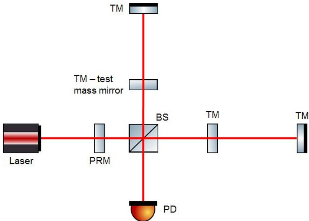
**Figure 1.** Basic interferometer setup for LIGO/Advanced Virgo. PD operating on the dark fringe will detect a phase difference between the light of each arm.
