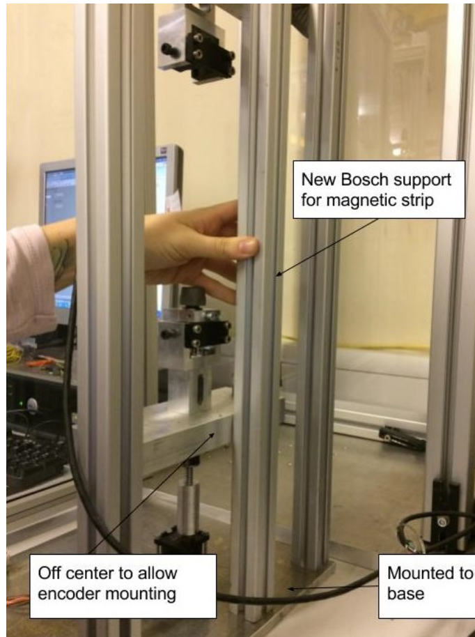
Figure 2.2: Image showing where the third Bosch bar was planned to be installed.
