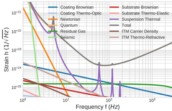
Fig. 13: Optimized noise curve of ET for a dual 1.4 solar mass binary system
