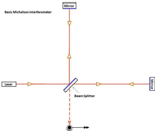
Fig. 1: Diagram of the basic Michaelson Interferometer
