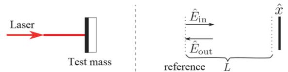
Fig. 3: Diagram of the propagation of the electric field through free space and its reflection off of a moving mirror
