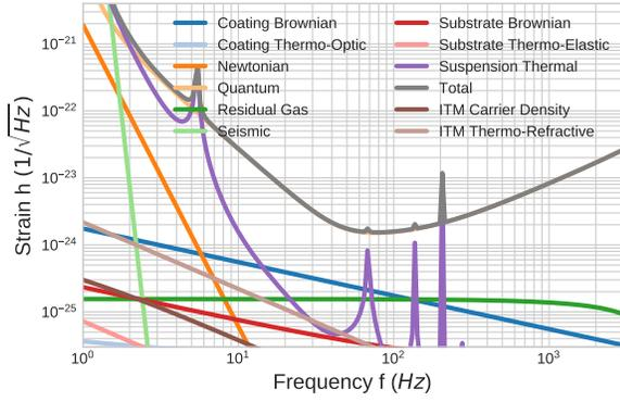
Fig. 12: Optimized noise curve of ET for a dual 25 solar mass binary system
