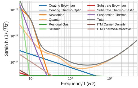
Fig. 10: Optimized noise curve of Voyager for a dual 1.4 solar mass binary system
