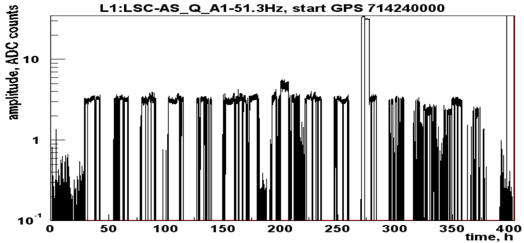
Figure 10. Amplitude of the 51.3 Hz calibration line for the S1 run data.
