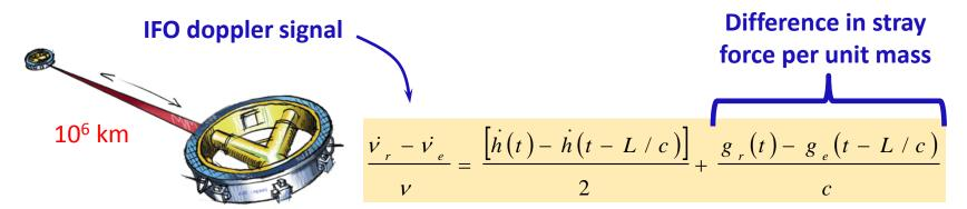
LPF as a differential accelerometer (2 TM in 1 SC)
