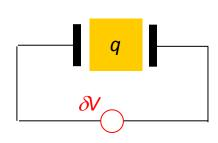
$$F_{x} = q \left\langle E_{x} \right\rangle = -q \Delta_{x} \left[ \frac{1}{C_{TOT}} \left| \frac{\partial C_{x}}{\partial x} \right| \right] \propto \frac{1}{\text{gap}}$$
