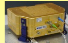
Reference Laser Head (RLH) - with Reference Cavity
