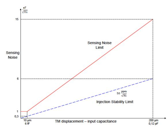
Requirement for the sensing noise in High Resolution mode
