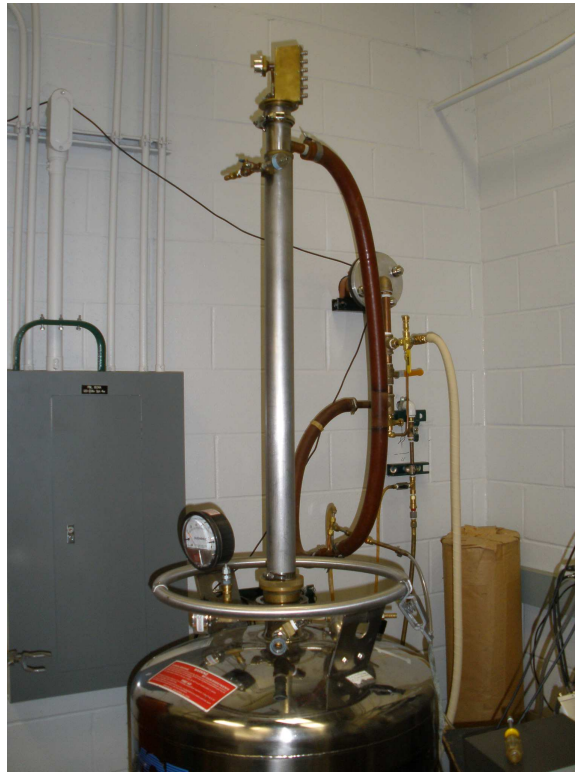
Figure 1: Dipstick in helium dewar: The long tube is the dipstick, which is shown inserted into the helium dewar at the bottom. When experiments are underway, the tube is fully inserted. All experimental devices are contained inside the metal sheath of the dipstick.
