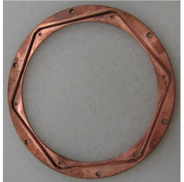
Figure 4 – Design for the open ‘lid’ of the detector (Left), machined lid (Right). The lip secures the detector and the inner screws mount the ‘lid’ to the detector. The outer screws secure the rods which suspend the piezoelectric motor above the detector.
