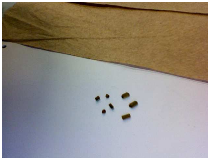
Figure 5: DTN crystals used in the experiment. Diameter of \sim 1/4 in. long and \sim 1/8 in. thick.
