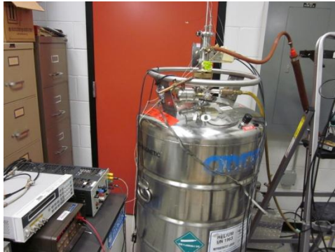
Figure 3: The suckstick inside the liquid helium dewar attached to electronics.
