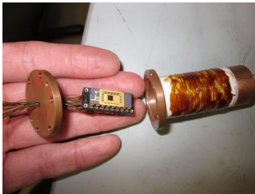
Figure 1: Pressure sensors next to the copper cell which has resistance wire wrapped around and coated in varnish.
