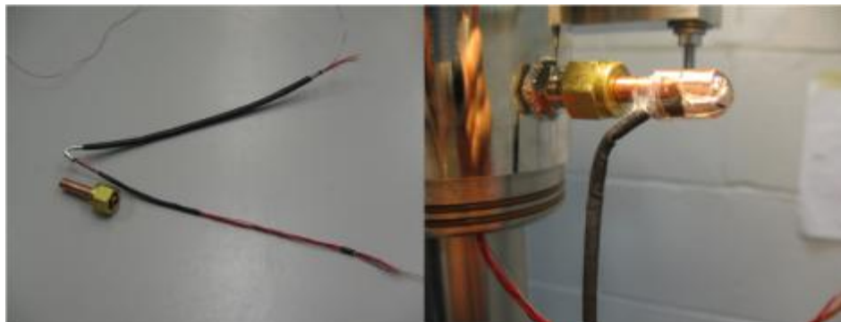
Figure 5. Feed-through components before assembly (left panel) and mounted feed through (right panel)
