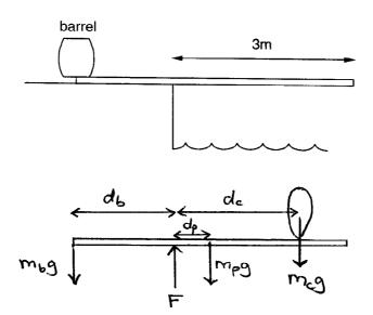
At the point where the plank becomes instable, the force of the deck acts only at the edge, which is the (potential) pivot point.
