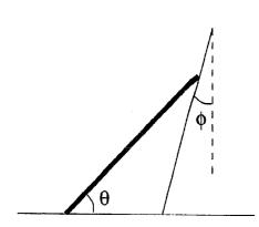
Since the wall is frictionless, the force it exerts on the ladder is normal to the wall.
