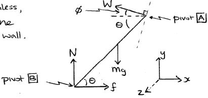
$$\begin{array}{lll} \Sigma F_{x} = 0 \Rightarrow & f - W \cos \phi = 0 & 0 \\ \Sigma F_{y} = 0 \Rightarrow & N + W \sin \phi - Mg = 0 & 2 \\ \Sigma T_{z} = 0 \Rightarrow f L \sin \theta - N L \cos \theta + Mg \frac{1}{2} \cos \theta = 0 & 3 & \text{closet } \boxed{A} \\ & \underline{\sigma} \quad W L \sin (\theta + \phi) - Mg \frac{1}{2} \cos \theta = 0 & \underline{G} & \text{closet } \boxed{B} \end{array}$$
