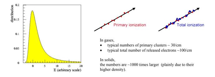
Landau fluctuations (Landau tail) correspond to rear large energy transfers from the incident particle to atomic electrons. Such electrons are called  $\delta$ -electrons. They typically can cause additional ionization, leading to a cluster of a few electrons.
