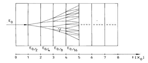
The picture above illustrate a simplified model of an electromagnetic shower. Only bremsstrahlung and pair production processes are considered. For simplicity, we will assume  $\lambda_{pair} = X_0$ .
