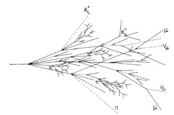
High energy collisions of hadrons typically result in prolific production of pions, the lightest particles made of quarks. Strong interactions of a kind  $pion + p \rightarrow k pions + p$  will, therefore, naturally lead to a hadronic cascade similar in many respects to an electromagnetic shower produced by electrons and photons. The main differences will be in a) mean free path between collisions;
