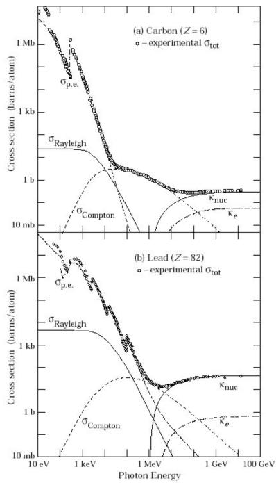
Total photon cross section  $\sigma_{tot}$  in lead, as a function of energy:
