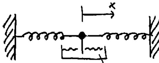
damping through viscous liquid
