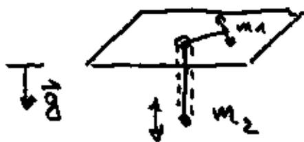
two masses, connected by thread
