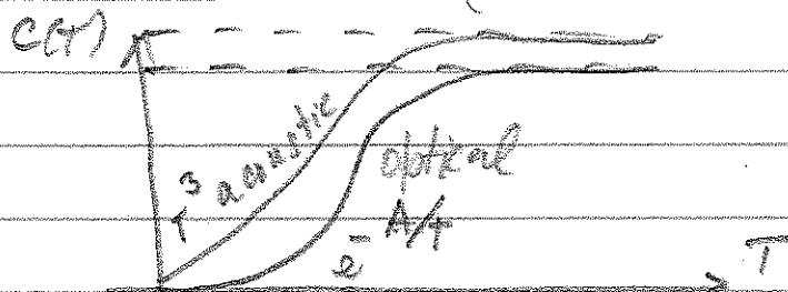
c) For  $T \gg \hbar \omega_0/k_B$ , optical phonons' contribution to  $C(T)$  is comparable with that of acoustic ones. For  $T \ll \hbar \omega_0/k_B$ , the optical phonon contrib. is exponentially small.
