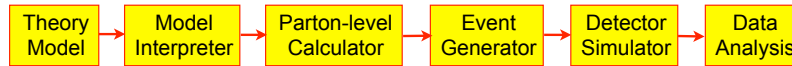
Fig. 1. The main steps in the simulation chain connecting particle theory to a collider experiment.
