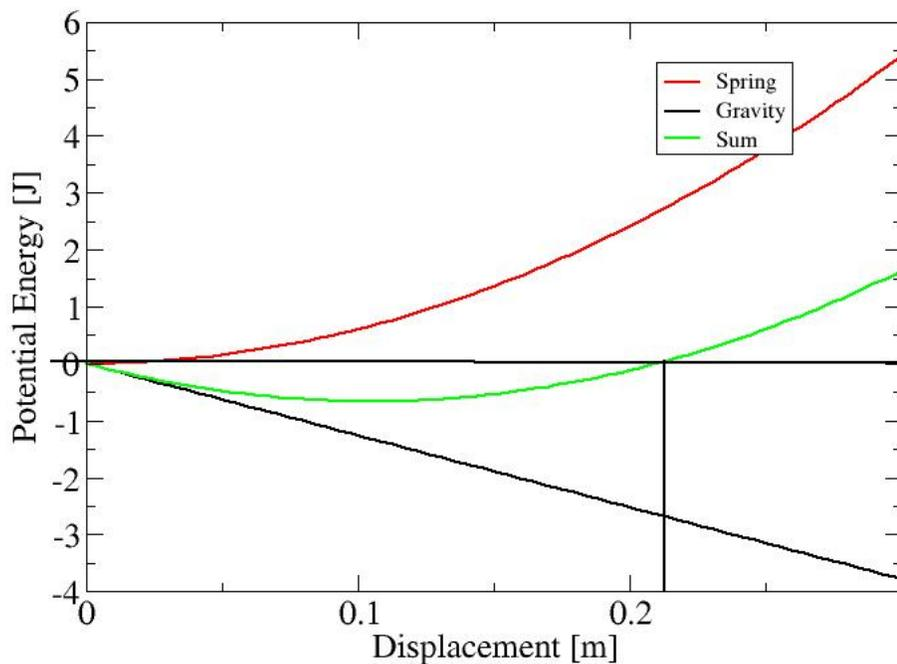
Gives us the turning point and also the stable equilibrium point where it would come to rest if friction or drag slows the motion down.
