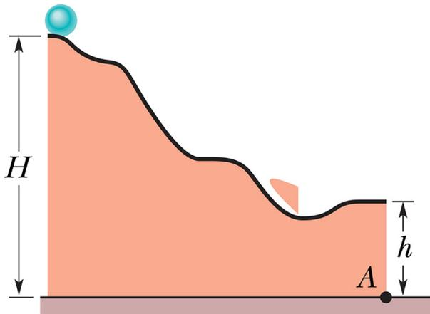
Smooth roll from Height  $H = 6.0$  m to height  $h = 2.0$  m. How far from  $A$  does the ball land?
