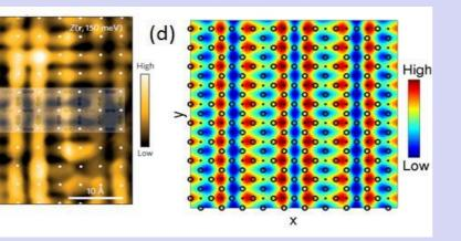
(a), (b) s, s' and d-form factors in BSCCO-2212 vs. STM bias: (a) experimental results from Hamidian et al, Science (2015) (b) Theory of Choubey et al, NJP (2017). (c), (d) conductance maps: (c) BSCCO-2212 cleaved surface (white dots represent the positions of Cu atoms); (d) Theoretical LDOS
