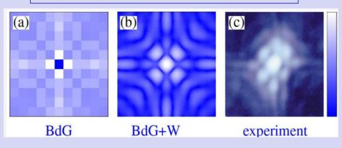
Calculation of Zn impurity in BSCCO-2212 (Kreisel et al PRL 2015): a) traditional Bogoliubov-de Gennes (BdG) solution; (b) BdG+W approach from Choubey et al PRB 2014; (c) expt. from Pan et al Science 2001.
