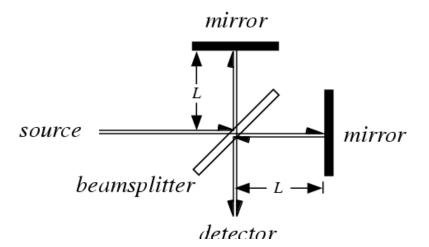
The interferometer was designed to detect the delay in the arrival of a light pulse due to the "ether wind" along the direction of the Earth's motion through the ether.
