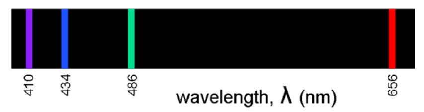
Bohr model  $E_{mission} = E_i = -\frac{R_y}{n_i^2}$   $\Delta E = E_i - E_f = hf$   $E_f = -\frac{R_y}{n_f^2}$   $-\frac{R_y}{n_i^2} - (-\frac{R_y}{n_f^2}) = hf$   $R_y(\frac{1}{n_f^2} - \frac{1}{n_i^2}) = hf$   $= \frac{e^4 m}{8s_i^2 h^2}(\frac{1}{n_f^2} - \frac{1}{n_i^2})$
