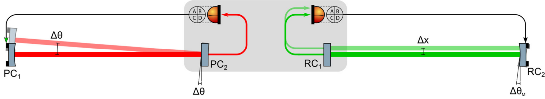
Fig. 5. Control architecture for maintaining spatial overlap. The QPDs on the COB monitor the position of the cavity eigenmodes on the cavity mirrors PC_2 and RC_1 . These signals are used to align the cavity mirrors at the end stations PC_1 and RC_2 . The aligned configuration is shown as the solid image in the foreground, while examples of the potential alignment errors are shown as transparent images in the background.
