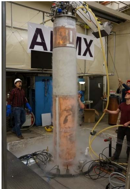
Fig. 1. Left: The ADMX insert, containing (bottom to top) the resonant cavity, SQUID amplifier and cryogenic post amplifier inside a bucking coil to maintain zero field at the SQUID, and helium reservoir is being removed from the magnet. Most of the 7 T magnet is below floor level. Right: Conceptual design of a 25 T HTSC magnet in which 2 to 16 cavities would be located to enable searches in the 3 to 12 GHz range.
