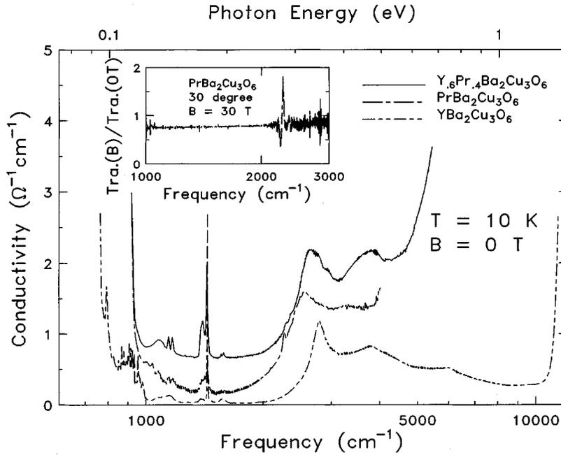
FIG. 1. The 10 K optical conductivities for  $\text{PrBa}_2\text{Cu}_3\text{O}_6$  (short-long dashed line),  $\text{Y}_{0.6}\text{Pr}_{0.4}\text{Ba}_2\text{Cu}_3\text{O}_6$  (solid line), and  $\text{YBa}_2\text{Cu}_3\text{O}_6$  (short-short-long dashed line). The inset shows the ratio of the 30 T to the 0 T transmittances  $T(30\text{ T})/T(0\text{ T})$  for  $\text{PrBa}_2\text{Cu}_3\text{O}_6$  in the  $30^\circ$  configuration ( $T=10\text{ K}$ ).
